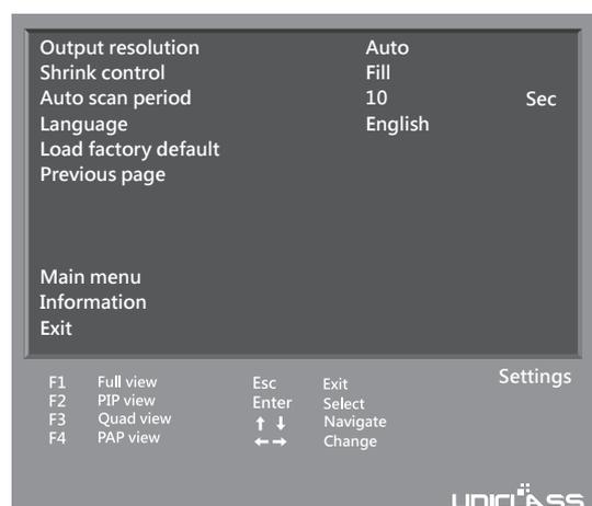
Press  $\uparrow$  /  $\downarrow$  on keyboard or  $\blacktriangle$  /  $\blacktriangledown$  on the front panel of unit to move cursor, press  $\leftarrow$  /  $\rightarrow$  or  $\blacktriangleleft$  /  $\blacktriangleright$  to select the desired option, and then press **Enter** or **OSD menu** button to confirm.
